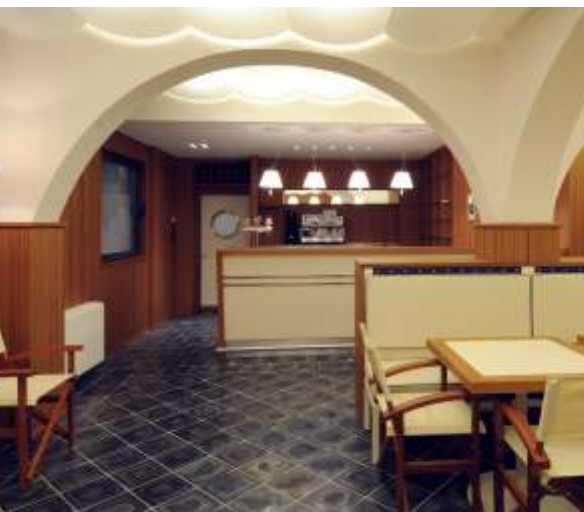
A tile made of cast basalt size 200/200 or 250/250 mm Comes from molten basalt of temperature around 1300°C / 2372°F
